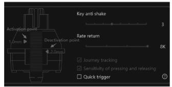
Set activation point (1.0mm), press the key to set point (1.0mm) to activate the key. Set deactivation point (2.0mm), release the key to set point (2.0mm) to deactivate the key.
