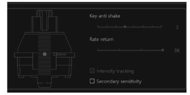
Press the key to set point (2.0mm) to activate the key. Release the key to set point (2.0mm) to deactivate the key.
